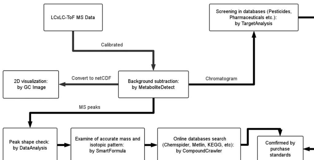
**Figure 1.** Workflow of LC × LC-ToF MS non-target analysis and suspected screening in environmental research, as developed in this study.
