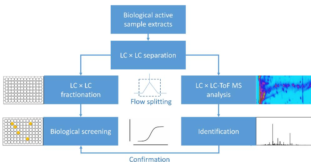
**Figure 2.** The EDA workflow developed in this study using LC  $\times$  LC for fractionation into 96 well plates.
